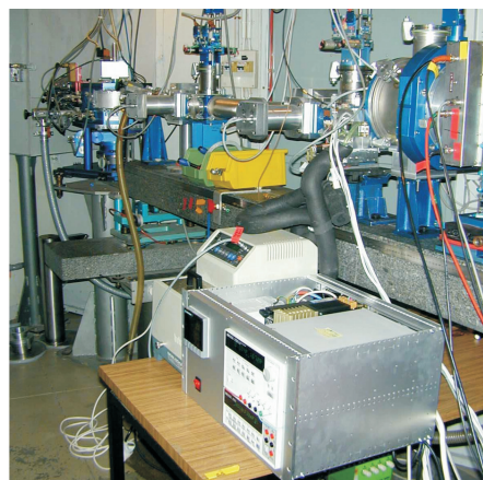
Fig. 2 Photo of one of the calorimeters installed on the bench D24 of LURE with a single long position sensitive detector
